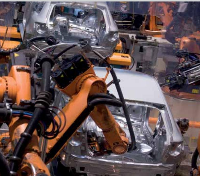
In automobile production, robots coat body parts with a fluid wax preservation coating
