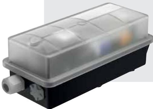
**templine®-B** Electronic temperature controller with integrated temperature limiter (safety temperature limiter). PI control characteristic, system deviation +/- 1K. Sensor input: PT100, two/three conductor technology. Switching capacity: 1360 VA/ 6A.
