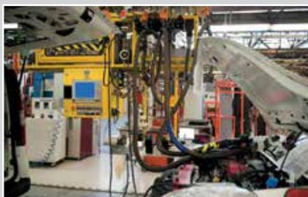
Wax-conveying hoses, heating capacity 60-120 W/m. Heating with minimized tolerances to guarantee extremely uniform consistency
