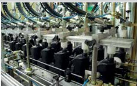
Co-extruding plastics. Conveying fluid plastic granules to the extrusion mould in heated hoses. Optionally: Temperature-monitored extrusion head with integrated sensor in the mould head. Heating capacity: 60-140 W/m
