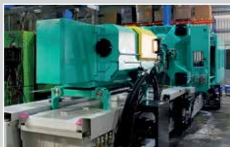
CNC-controlled injection moulding machine. Temperature-controlling the plastic and adhesive in the heated hose during manufacture of housing parts (PA, TPE, EVA). Temperature of medium: +90°C to +180°C
