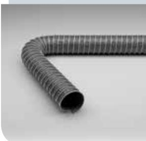
PVC coated Polyester Suction & Blower Hose, antistatic, surface resistance  $R_0 < 10^9$ , extra strength outer wall, good resistance to mechanical damage, lightweight
