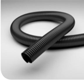
PU Suction & Transport Hose, electrically conductive  $R_0 < 10^4$ , flame-resistant, highly abrasion resistant, oil/petroleum-proof, improved pressure and vacuum characteristics, smooth inside for optimum flow
