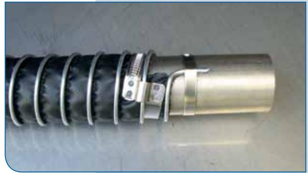
As is shown in images 8 - 9, the metal clip profile sits on the pipe and is fixed in place by the separate clamp, metal on metal. This type of connection is recommended. Other methods of grounding are also possible, however, we would like to point out the following:
