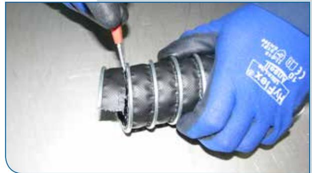
2. Cut the wall material to approx. 30 mm along the metal clip helix spiral.
