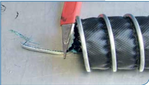
6. Remove any remaining material from the metal clip profile.
